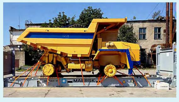
**In-gauge cargo** means that the dimensions of the cargo are smaller, or equal, to the container dimensions. Cargo more than 244cm wide on a flatrack is considered out of gauge.
