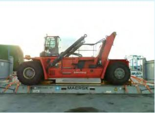
The simple top over lashings can be used as well, but we do not recommend it to be used alone. Please do combine it with one of the above methods. For calculation purpose, use the system of MSL figures provided by the lashing material manufacturer
