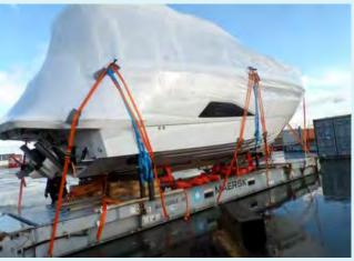
As for top-over lashings, a calculation must be made using the applied tension values as supplied by the manufacturer, along with friction and acceleration factors.
