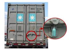
Affix the container seal at the bottom bar but with the head facing upward
