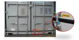
This seal placement is recommended to avoid possible operational constraints and potential issues related to seal damage/breakage caused by rough handling at berth or terminal, or by concussion or friction with rail wagon clam/guard during loading where the container seal has direct contact. Damage to the container seal exposes your shipments to safety risks, which may also lead to delivery delays and additional cost.
