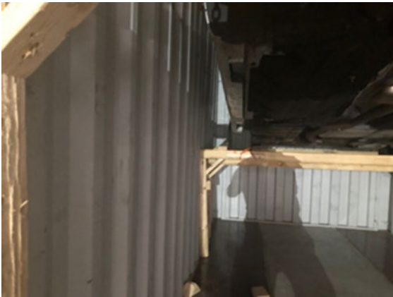
Fig 3. Suspending vehicle from upper rings
