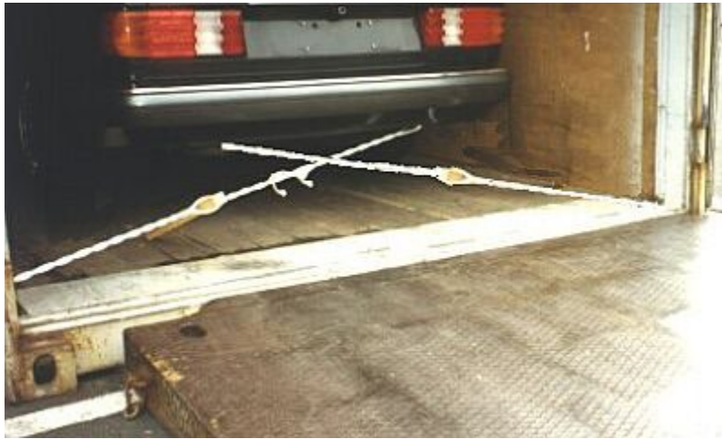
More favorable lashing arrangement from two lashing points
