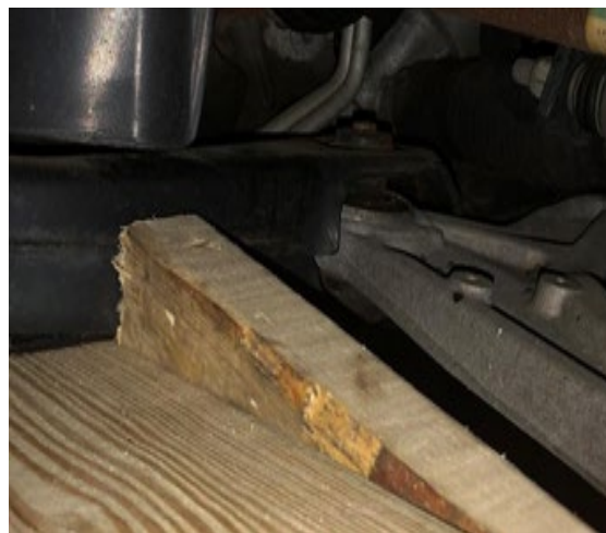
Fig 5 and 6. Axel lashed and blocked to cradle to prevent swaying
