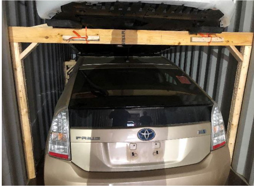
Fig 7. Second vehicle stowed under the first.
