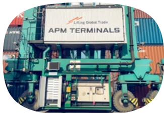
Hybridisation of 2 Rubber Tyre Gantry Cranes in Gateway Terminals India, contributing to >50% of fuel and emission savings
