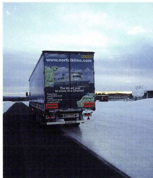
A Norfolkline trailer on a split friction part of the track, where one side is heated asphalt and the other is polished ice.
