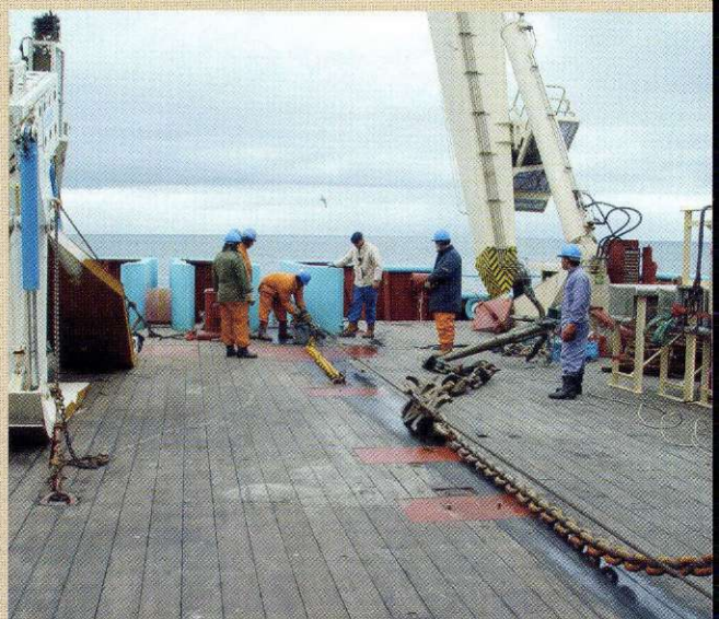
The working deck with the 20-ton heavy plough to the left. The last scrap cable is taken on board after cleaning of the cable route.
