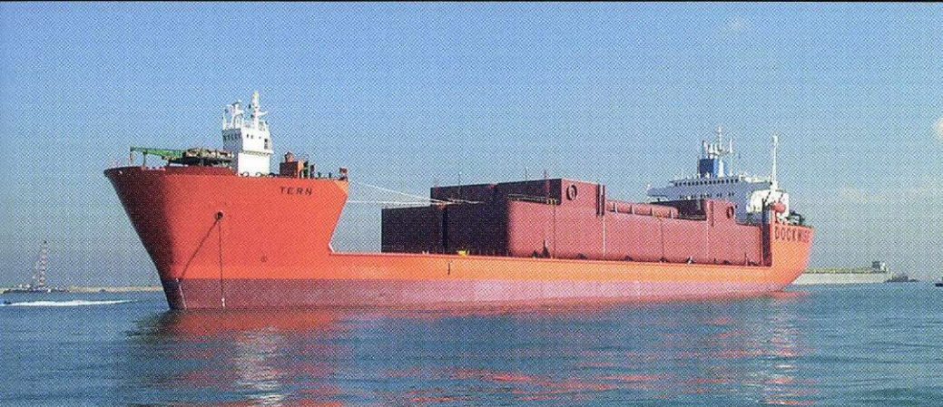
The two pontoons were transported on a heavylift vessel from Singapore to Kerch, Ukraine where they were offloaded and towed the remaining distance to the Azerbaijani capital Baku. Each pontoon weighs 1,500 tonnes and is 90 metres long, 14 metres wide and 8.6 metres high.
