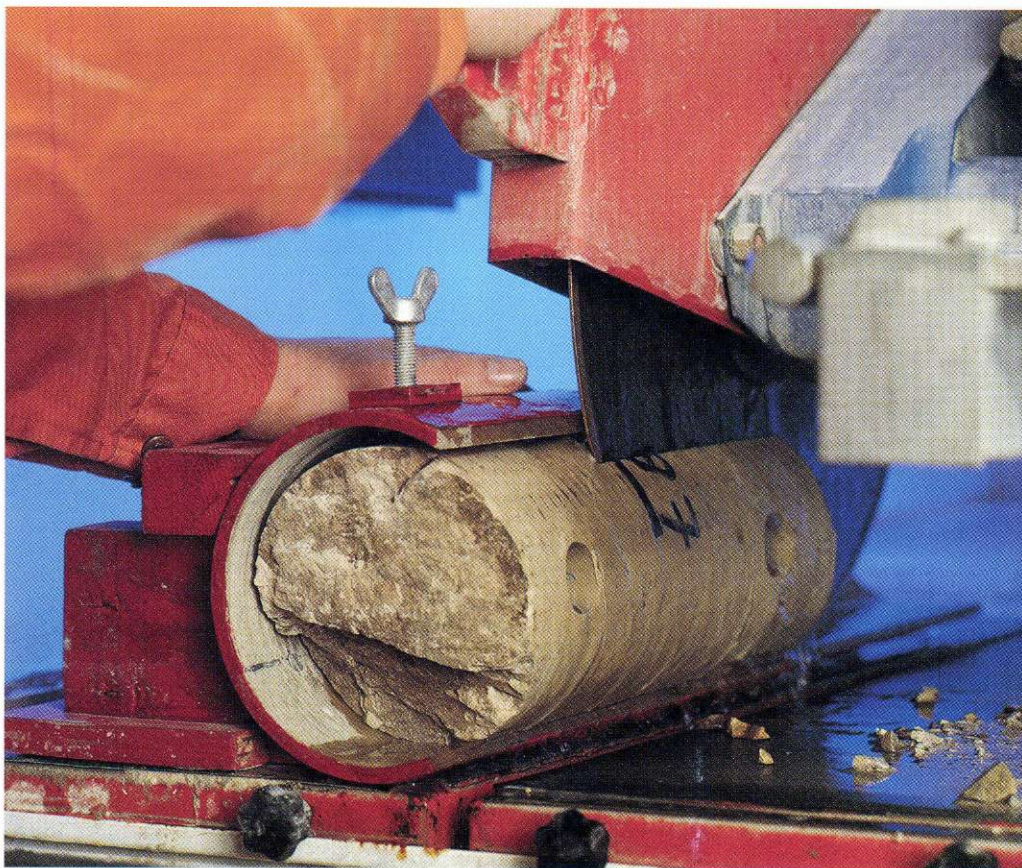
The core is cut through lengthwise.
