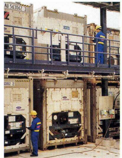
One of Brigantine's reefer technicians checking the temperature of a reefer container.
