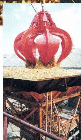
A tailormade 17 cbm orange peel grab discharging wood chips to a "hopper" in Bellingham.
