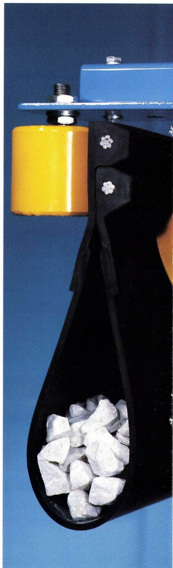
The closed conveyor belt, made in the form of a drop-shaped bag, was manufactured by A/S Roulunds Fabriker.
