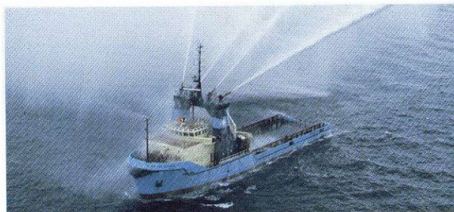
m.s. "MÆRSK CLIPPER" with fire-fighting equipment Built: Dannebrog Værft A/S, Lindø
