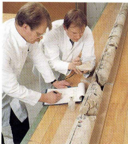
A detailed description is made of all geologic features observed in the cores. Lab Supervisor Søren Pedersen and Geologist Mike Yusas examine a core from the Kraka Field to record and fossils, fractures, oil staining etc. This information is used to predict the size of the oil reservoir.
