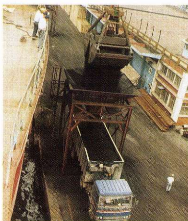
The mobil hopper is placed on the quay and, by the means of the vessel's cranes and grabs, the goods are discharged onto the truck.
