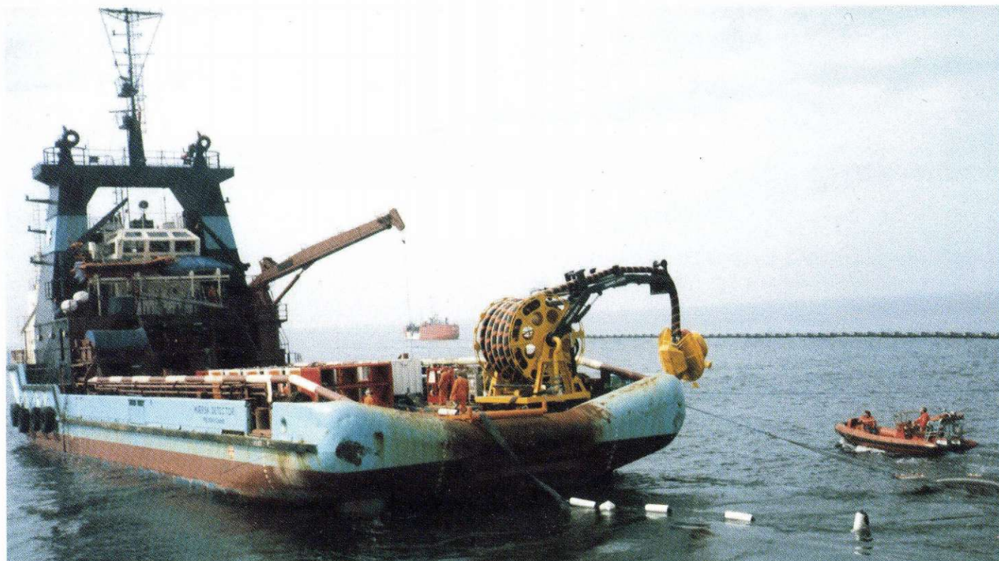
Frequent drills are carried out as practice in controlling oilspills. Shown in the picture is the supply vessel "MÆRSK DETECTOR" with an oil suction unit on the quarterdeck. In the background the oil booms which have been laid out can be glimpsed.
