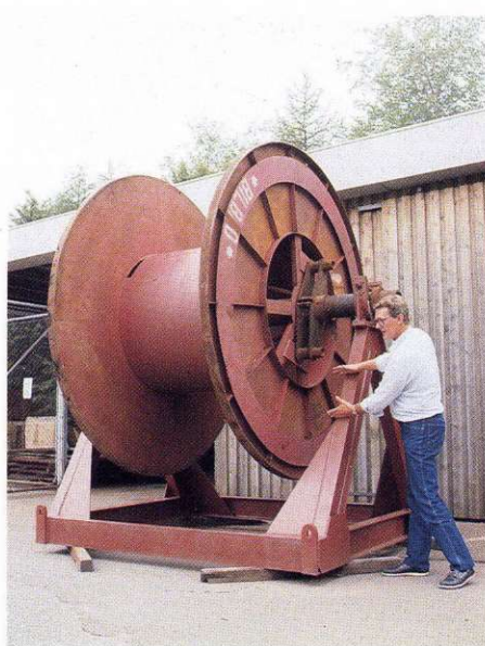
The Workshop Training School's leader, Kurt Hansen, explaining how one of the wire rollers which the school has constructed for use on supply ships functions.
