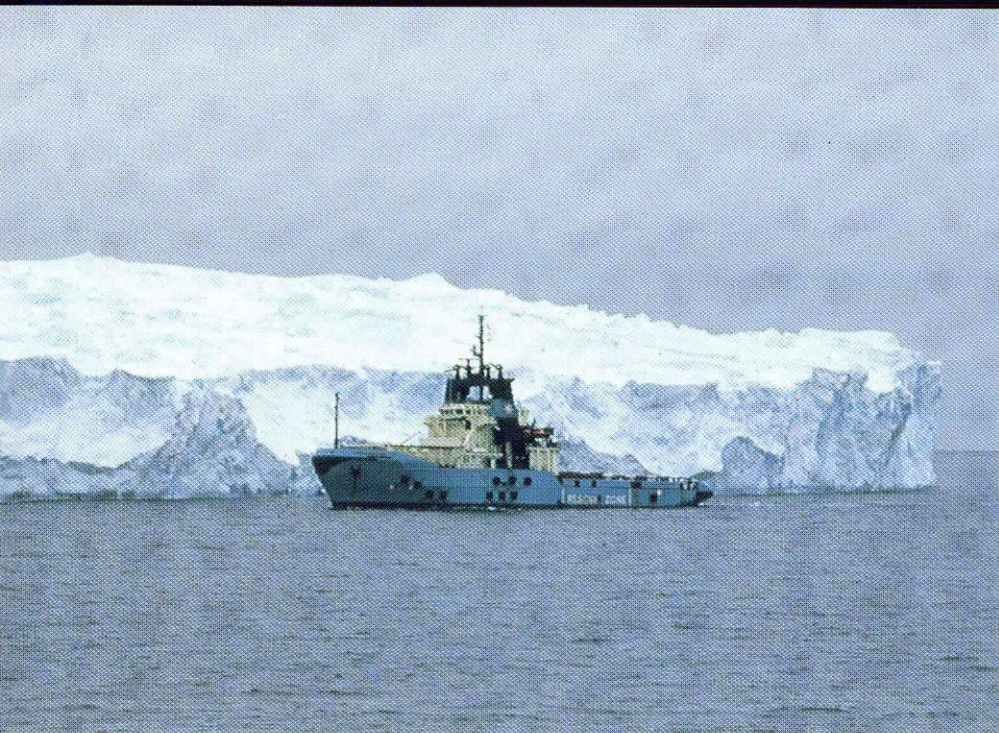
The "MÆRSK MASTER" sailing around an iceberg off Antarctica, paying out a floating tow line to lasso the berg and tow it away.
