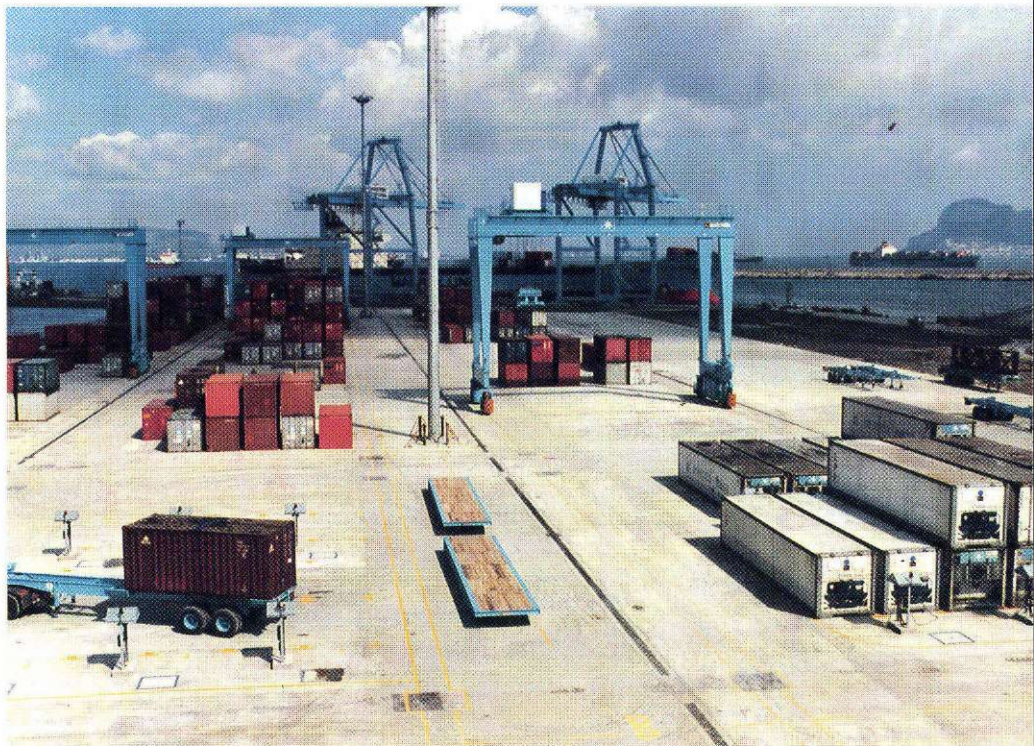
The three transtainers each capable of spanning stacks of containers six wide and five high.
