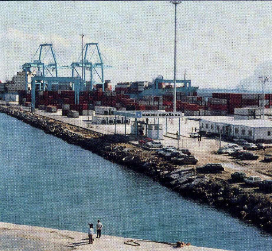
The three transtainers each capable of spanning stacks of containers six wide and five high.
