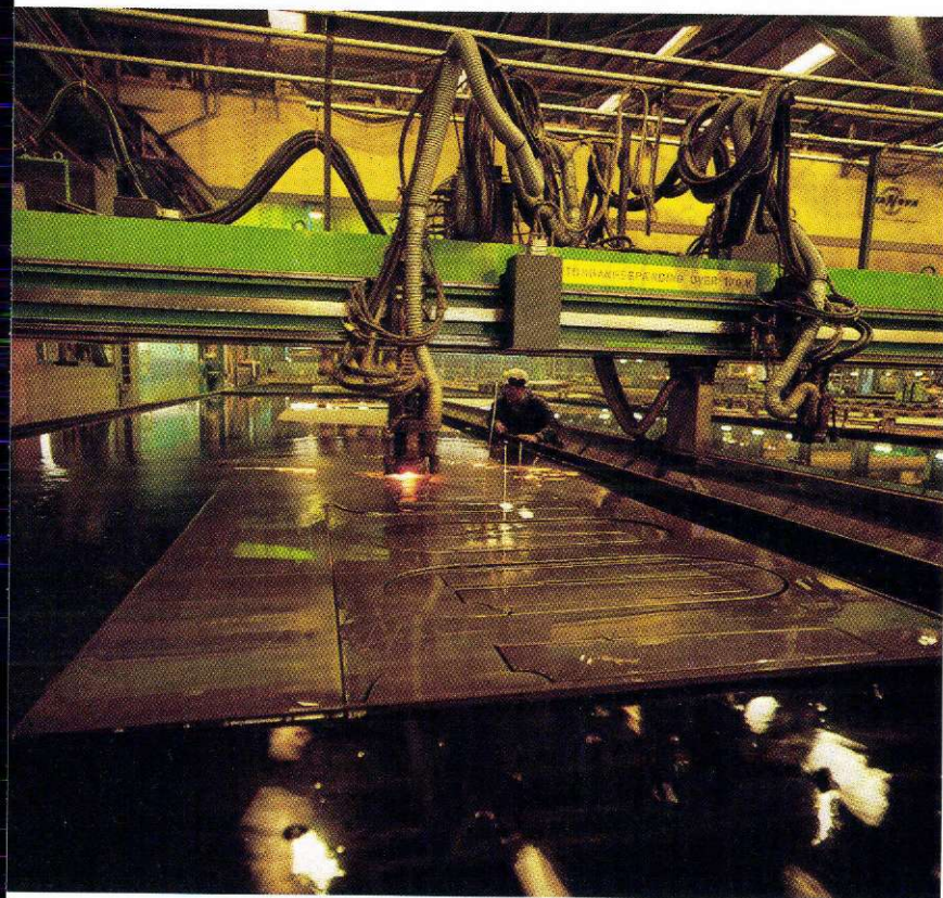
Computer-controlled cutting of steel plates.
