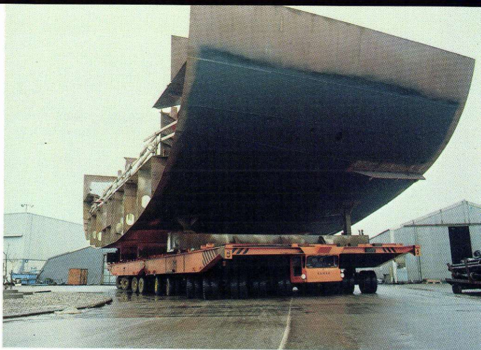
An automatic truck with 48 wheels, taking a completed engine-room for assembly in the Building Dock.
