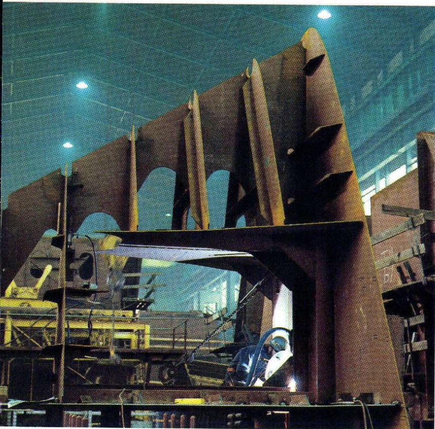
Welding the hull sections in the Assembly Hall.
