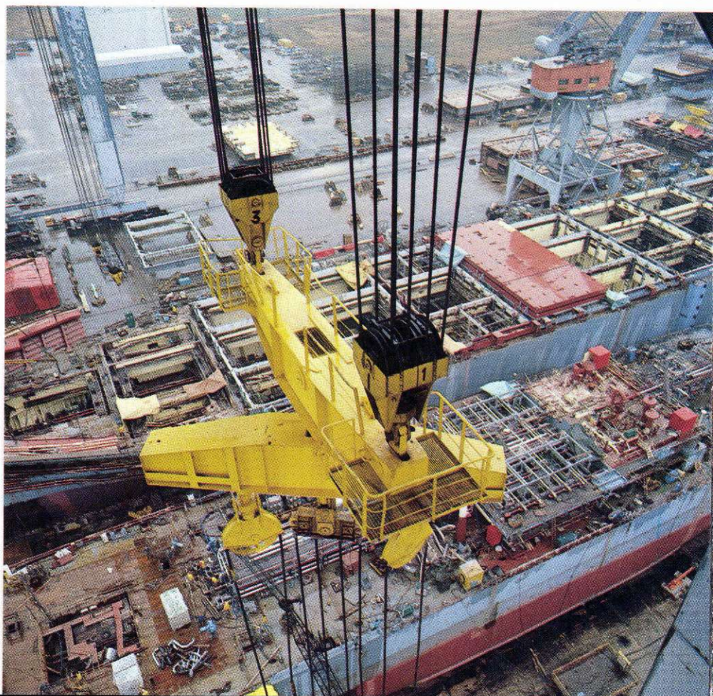
In the Building Dock a section is lifted into place by Lindø's gantry crane, lifting capacity 800 tons.
