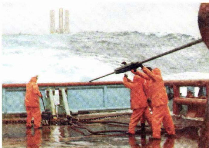
The 'protector', which is intended to save the towline from being chafed against the gunwale aft, is fixed. It was soon broken, however.
