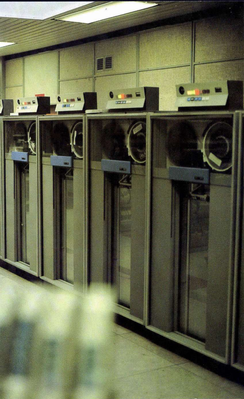
Magnetic-tape units. Magnetic tapes are used as back-up media and for the storage of large quantities of data that do not require on-line access.
