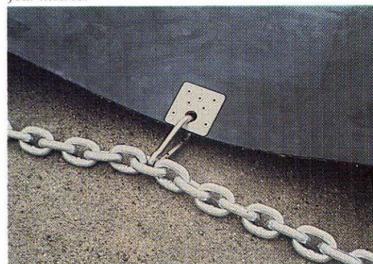
A ballast chain secures optimum position of the skirt under sweeping operations.
