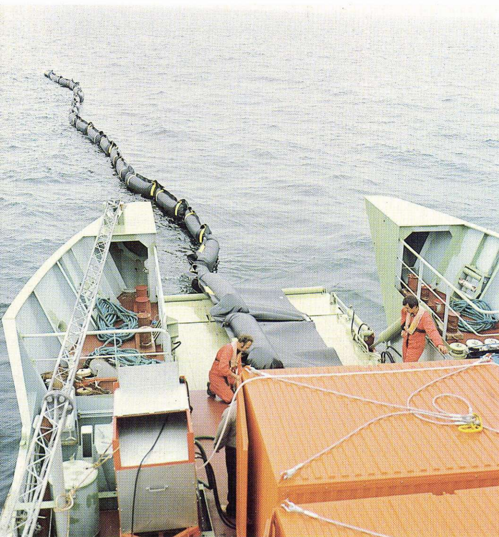
Roulund's anti-pollution oil boom, RO-BOOM, being deployed from m.s. "MARIE MILJØ", belonging to the Department of the Environment. The booms are kept and transported in containers, rolled on winders.
