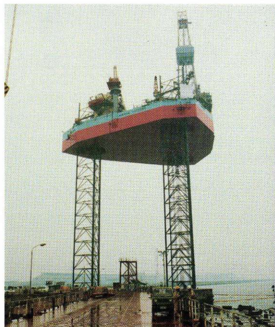
"MÆRSK VICTORY" at the yard in Japan. The legs are 123 metres long, and when they are stretched to extreme position, the total height of the rig is 164 metres.
