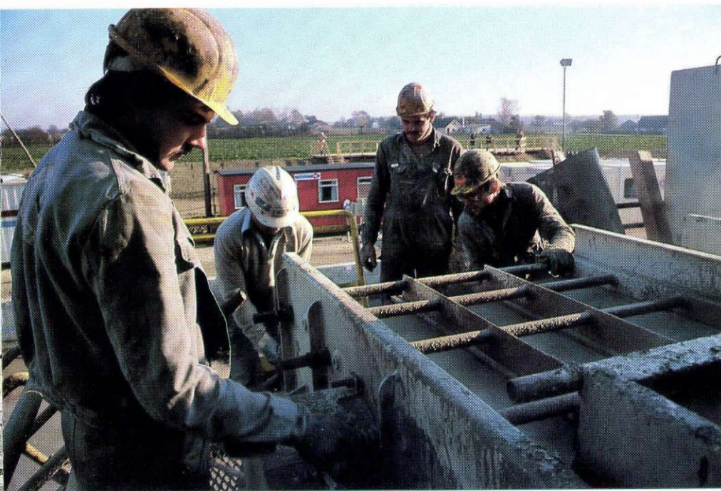
With drill-mud and cuttings reaching the surface, geologists will get the first signals of oil in the subsoil – if there is any oil.
