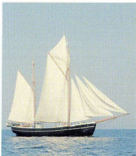
Baltic ketch "ANNA MØLLER" of Svendborg. 49 GRT. Built 1906 at Randers. This ketch has a Baltic transom stern and two polemasts. She carries three headsails, main gaff sail, and mizzen gaff sail. Above the main-sail she carries a gaff topsail.
