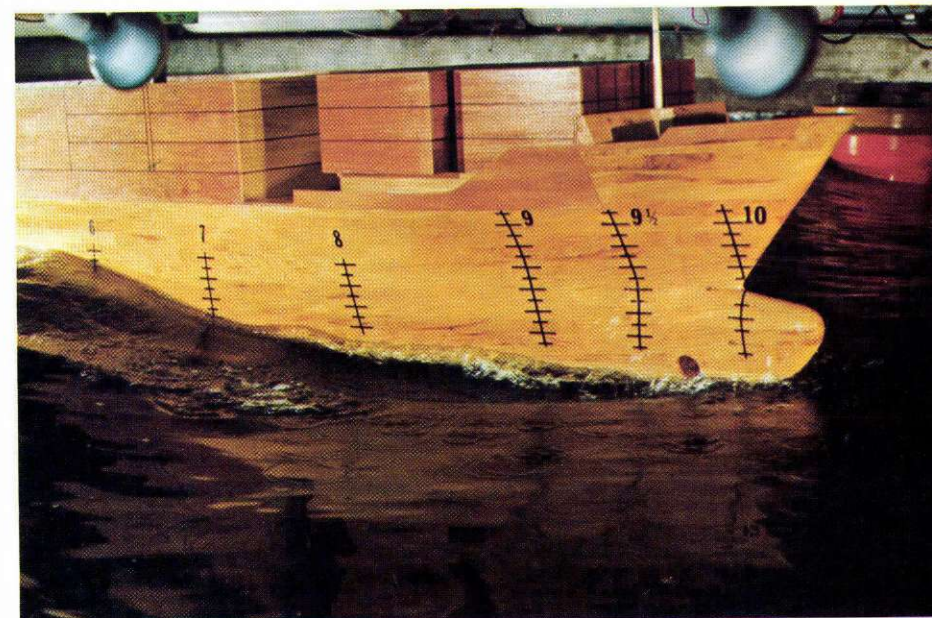
A couple of photographs taken during the tests of seaworthiness. The model is subjected to artificially created waves in the test tank at Skibsteknisk Laboratorium, Lundtofte.
